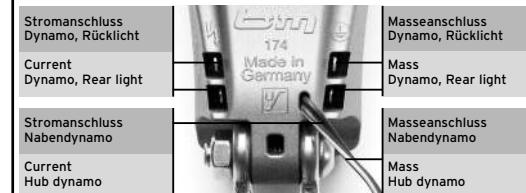
Use the preassembled duplex cable to connect the headlamp to the hub dynamo. Do not cut off the cable - just shorten it to the required length. Do not use the dynamo cable already provided on the bicycle.
